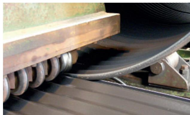
SPIROsol type SPM are produced through controlled mechanical cold deformation of round SPIROsol pipes with hydraulically cylinders to arch shape culverts.
