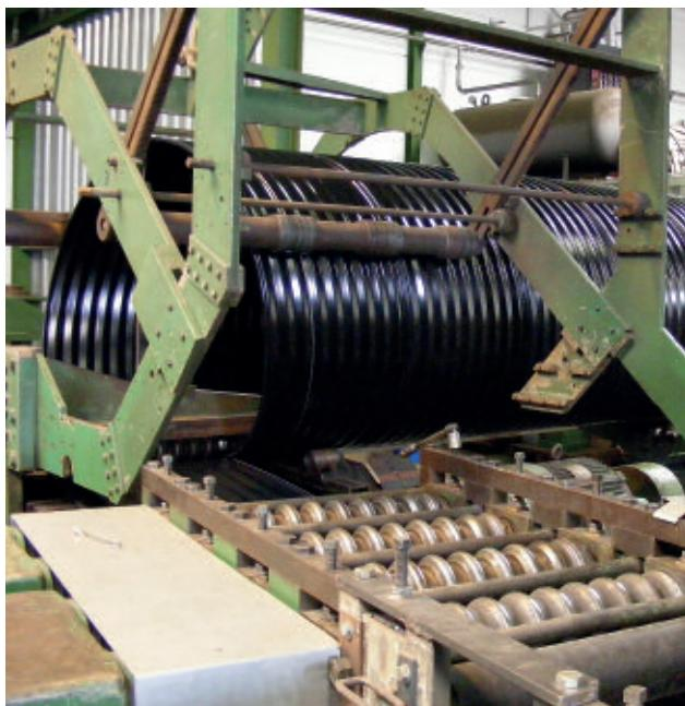
SPIROsol pipes are produced by cold forming of the strip. Initially the strip of steel will be mechanically formed with corrugations and after that bent/rolled in a diameter varies from 300 mm till 3000 mm. During forming of the pipe a lockseam is performed to provide a final strength and seal.
